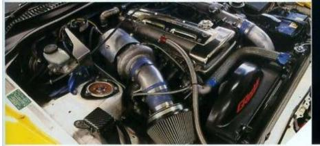
A LOT of aftermarket turbocharger upgrade kits for the 2JZ and 1JZ engines replace the stock twin turbocharger system with a big single one. Sounds odd, really, going back from two turbos to one, but the reality is that there are some very good reasons to go the single turbo route with these engines.
