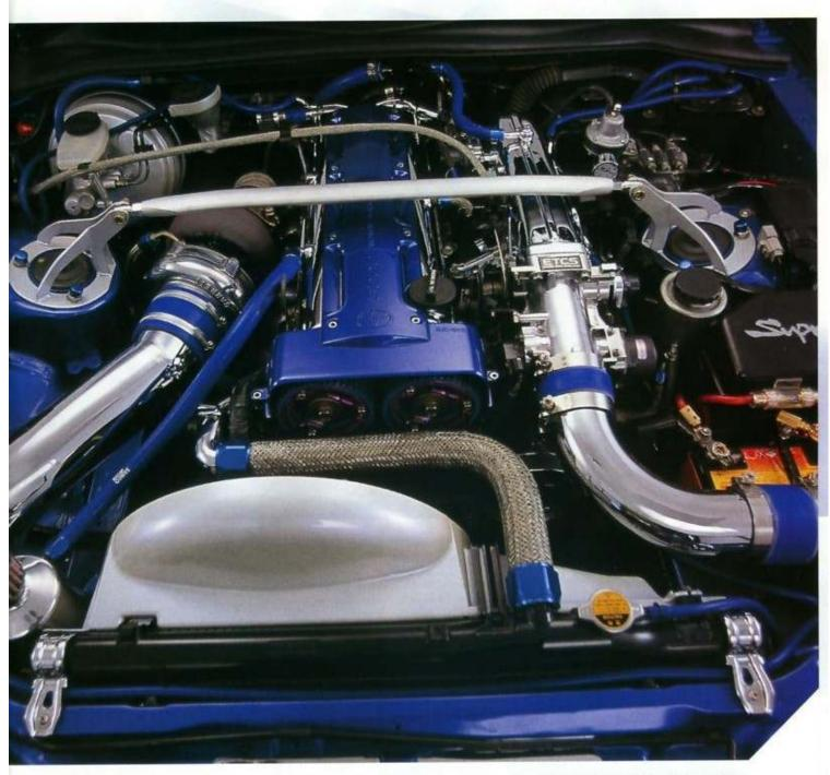
The basic 2JZ engine has a square layout, with a bore/stroke ratio of exactly 1:1. Its measurements are 86x86mm, giving 3000cc capacity, with a geometry identical to the much revered and super-expensive OS Giken three-litre race GT-R engine. The block casting itself bears no inherent weaknesses and, being made of cast iron, is superbly strong, if a little heavy.
