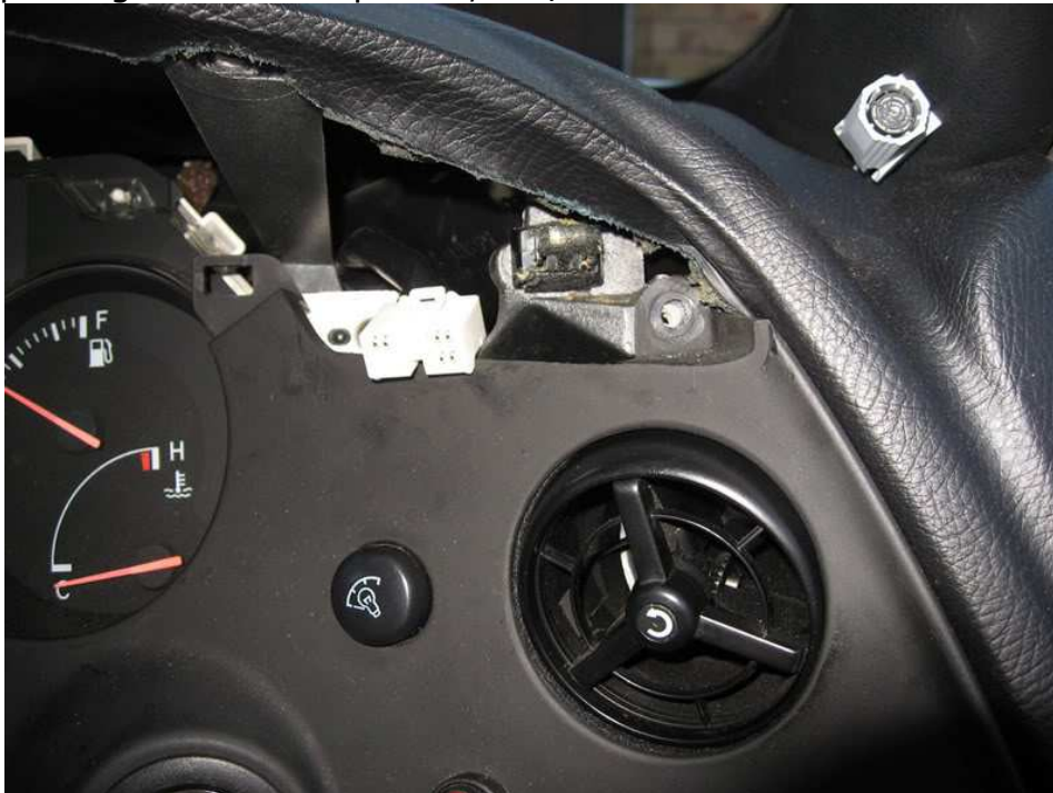
Top dash panel, right hand connector
