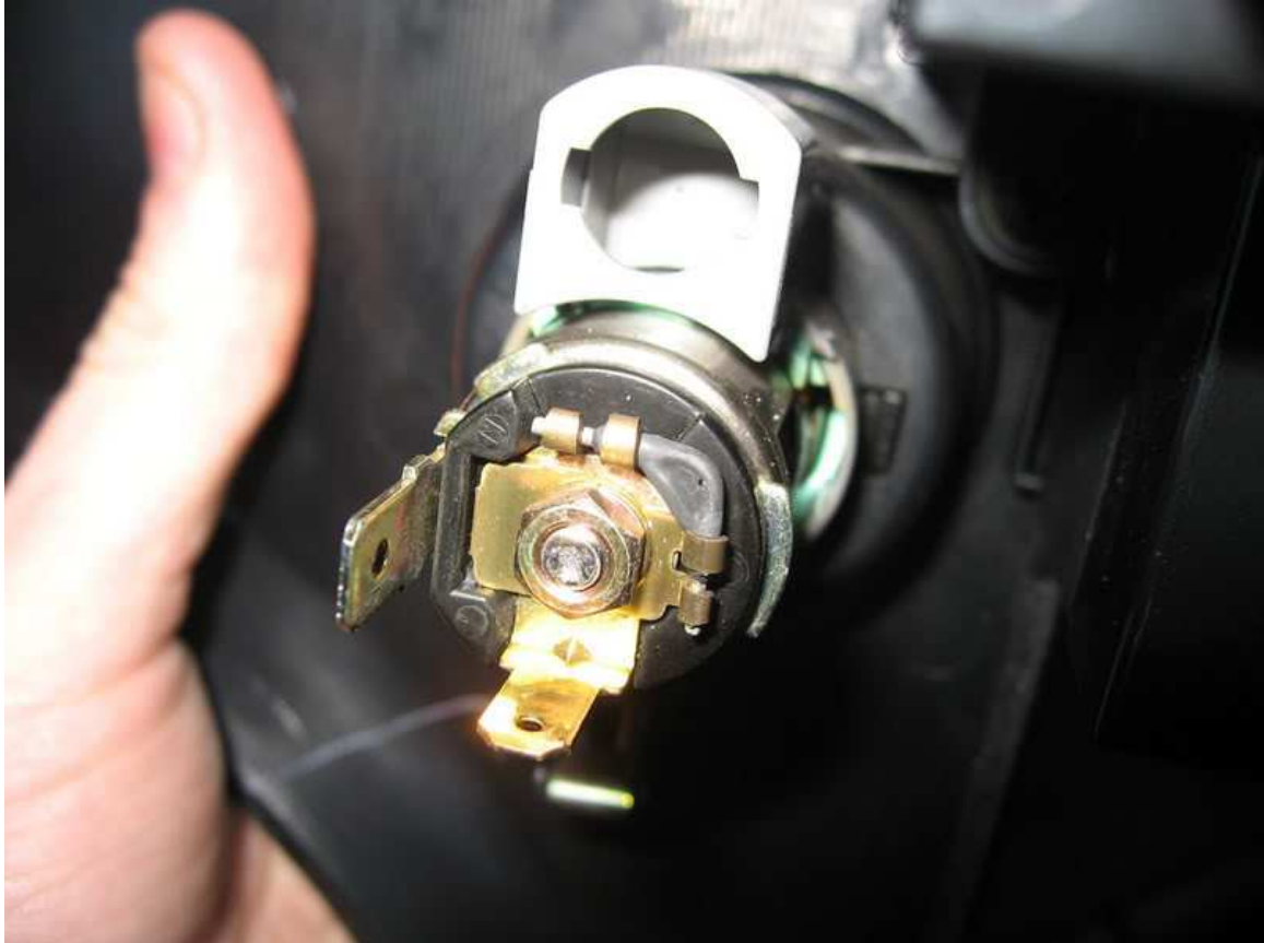
Cigarette lighter (rear) - shows L-shaped power connection and above that, the 'socket' for the light
