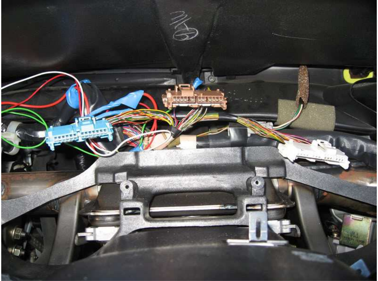
Instrument panel connectors - blue, brown, white
