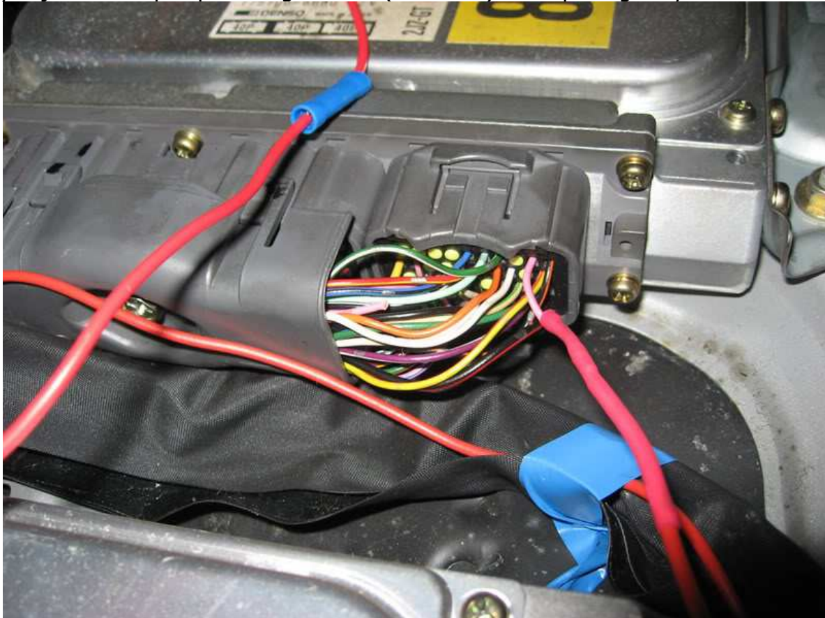
Modified ECU wiring - extension from Thor delimit chip spliced into the pink wire coming from pin 2, original loom end wire with bare end can still be seen
